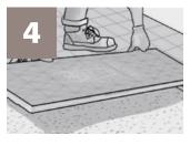
Make sure to install the Gator Base on the extended excavation area (total excavation should be 6" (15 cm) wider on each side than the final tiled area). • Start laying and staggering the Gator Base units ensuring Gator Base interlocks with the tongue & groove system.
