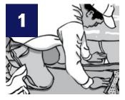
1 Spread EUROSTONE BOND with hard-bristle broom. Make sure the EUROSTONE BOND completely fills the joints. Do not use with other materials in the joints. Leave a layer of EUROSTONE BOND on the surface to aid in the vibrating and consolidation of EUROSTONE BOND into joints. 2
