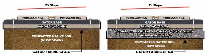
To use with 3/4 inch (20 mm) outdoor porcelain tile only. Sand or ASTM No. 9 Stone can be used under Gator Base panels.
