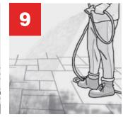
**9** Shower and rinse simultaneously, so as to eliminate any GATOR POLYMERIC SAND residue. Any residue should go directly into the paver joints. However, stop showering when you see water retention on the paver joints. Wait no longer than 2 to 3 minutes. Proceed to STEP 10.
