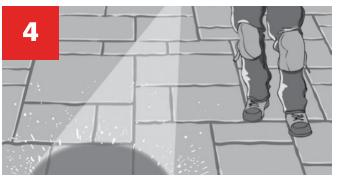
Shower for a minimum of 30 seconds for 30 sq. ft. (3 sq. m.) or until the SUPERSAND G2 repels the water and the water starts to accumulate on the joints.
