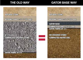
Adding a second layer 3/4 in (19 mm) of loose sand or ASTM No. 9 stone on top of the Gator Base for pavers or natural stones is also an accepted method of installation. Sand or ASTM No. 9 Stone can be used under Gator Base panels.
