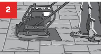
Vibrate the SUPERSAND G2 into the paver joints using a vibratory plate compactor. A rubber pad is recommended. A roller compactor is best for slab installation. Joints sand level must be at least 1/8 inch (3 mm) below top of paver's surface or 1/8" (3 mm) below the chamfer. It is best to compact in several directions to ensure there are no air gaps or voids in the joints. Repeat steps 1 and 2 to ensure joints are filled and consolidated. Narrow joints require more care to completely fill.
