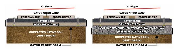
Sand or ASTM No. 9 Stone can be used under Gator Base panels
