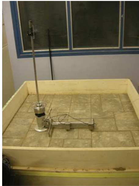
Figure 12. Light Weight Deflectometer
